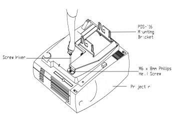
Using a screwdriver, secure the PDS-016 mounting bracket using three (3)
